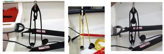
**Bowline**: Since the boat is for young kids, it is important to make sure the bowline is rigged and stored properly. The bowline dead ends at the mast step with a slip knot or tight bowline. If you use a bowline, make sure it's tight so it will not loop itself around the threaded adjustment rod. The boats are towed in a daisy chain configuration, so you also want to make sure there is a bowline on the bitter end of the line and it's coiled up and stuffed under the rail.
