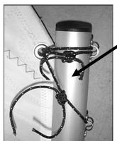
adjuster (halyard) is tensioned. It loops only once through the same throat eyelet, but at an angle to the lower eye strap. Instead of pulling this tie tight, adjust the loop so the top corner tie remains perpendicular to the mast when the sail is pulled upwards.
