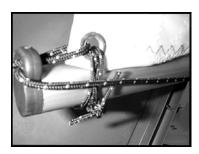
Finish up by tying the boom corner tie at the tack, followed by the loose intermediate boom ties (be sure to tie under the bridle or outhaul). Don't make the mistake of leaving off the clew corner tie and assume the outhaul will hold it down. This tie is just as important as all the others (see left pic).
