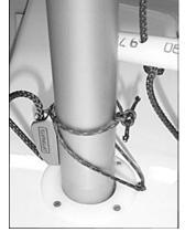
Immediately after stepping, the mast should be tied into the boat. The mast tie-in prevents the mast from coming out of the mast step cup and damaging the mast thwart in event of a capsize. The tie-in lines should be long enough to wrap around the mast, crossing over top of the vang cleat and securing in front with a square knot and a half. Test that the mast cannot be lifted out of the cup BEFORE the boat leaves the dock.
