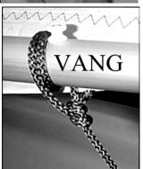
Next, add the **boom vang**. On the racing rigs, there might be a smaller line or wire that connects the vang adjustment line to the boom. On the club rig it is just a simple line and it can be secured to the boom with two half hitches or a doubled turn bowline. This will prevent it from riding over the vang peg toward the mast.
