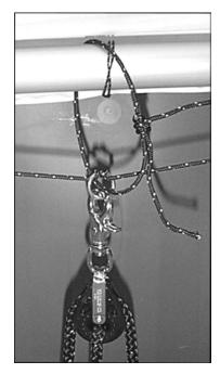
Once satisfied that the bridle it tensioned correctly, add the bridle preventer. The **bridle preventer** should restrict the bridle to pulling no more than 10 cm from the boom in the event it loosens. Tie the preventer with a sheet bend (a square knot would flip and loosen under tension).
